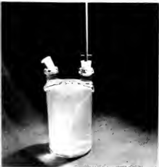
The pressure of one cork forces the other one out in a simple illustration of hydraulic action seen in "Harnessing Liquids."
