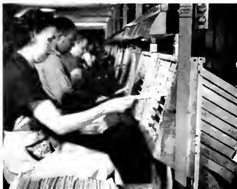
THE SESTAK MACHINE in action. Here separations are made on letters by state, railway post office or city, as indicated.
