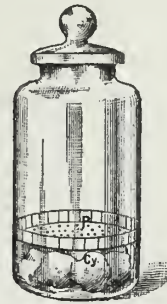
FIG. 46.—Cyanide-jar prepared for use: P , perforated cardboard; Cy , lumps of cyanide of potash.
