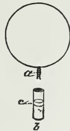
FIG. 45.— a , ring of metal tied with wire at a ; b , ferrule; c , plug put in before pouring in solder (Riley).
