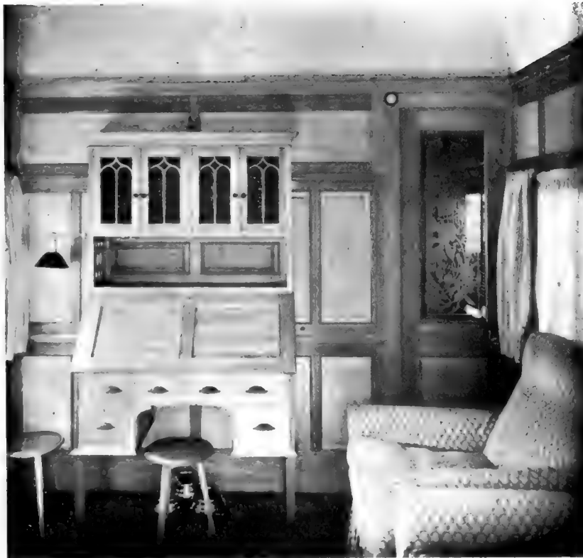
Spotted Gum Framing, Celery Top Pine Panels. Smoking-room, State Governor's Carriage, N.S.W. Government Railways.
