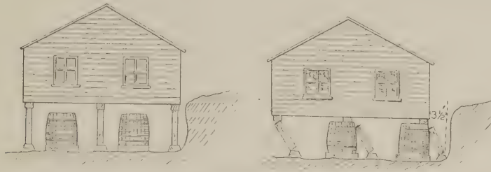
FIG. 56. — Section thru winery at Morrell ranch before and after the shock.
