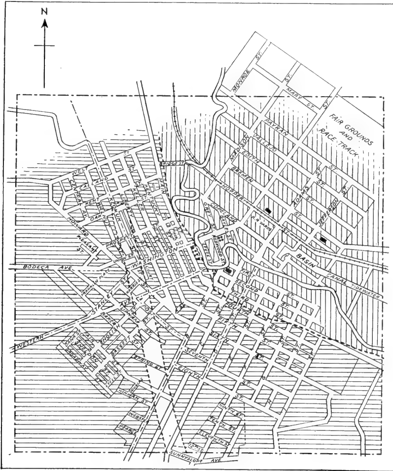
FIG. 64.—Distribution of intensity in Petaluma. Vertical lines represent area of low alluvial land, on which nearly all chimneys were damaged. Horizontal lines represent slopes underlain by rock, on which about half the chimneys were damaged. The solid black areas and dots represent exceptionally severe damage. The blank area enclosed by dotted lines represents a belt of practically no damage. By R. S. Holway.
