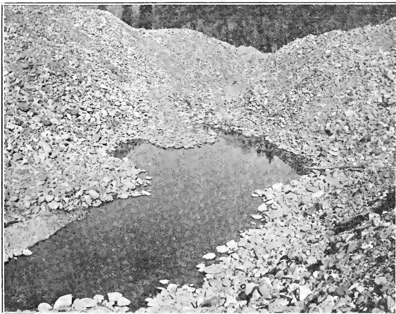
FIG. 43. The mining dredger is a menace to fish. The picture shows how completely the Trinity River was blocked by dredging operations in 1926. It is evident that no migratory fish could successfully pass such an obstruction during low water. Photograph by G. O. Laws.
