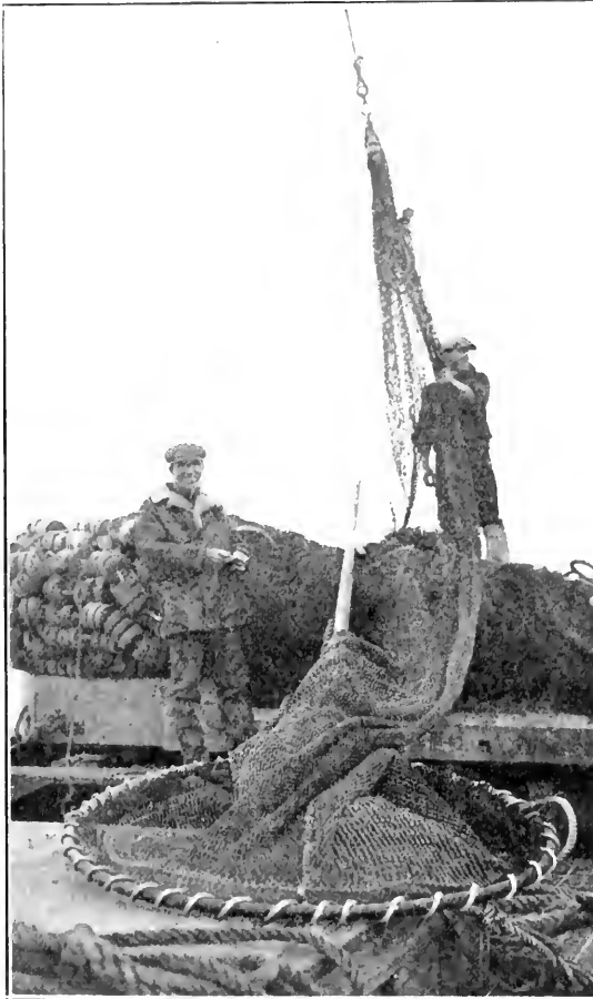
FIG. 40. Long bag dip net such as is used by purse seine boats for unloading catch from net into hold of boat. Note that the end of the bag is closed and fastened to hoisting rope, by means of which the net is emptied. Photo by J. B. Phillips, February, 1932.
