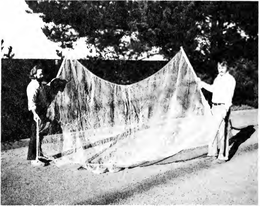
FIGURE 1. Net with dowels attached. Photograph by Kim McCleneghan, November 1976.
