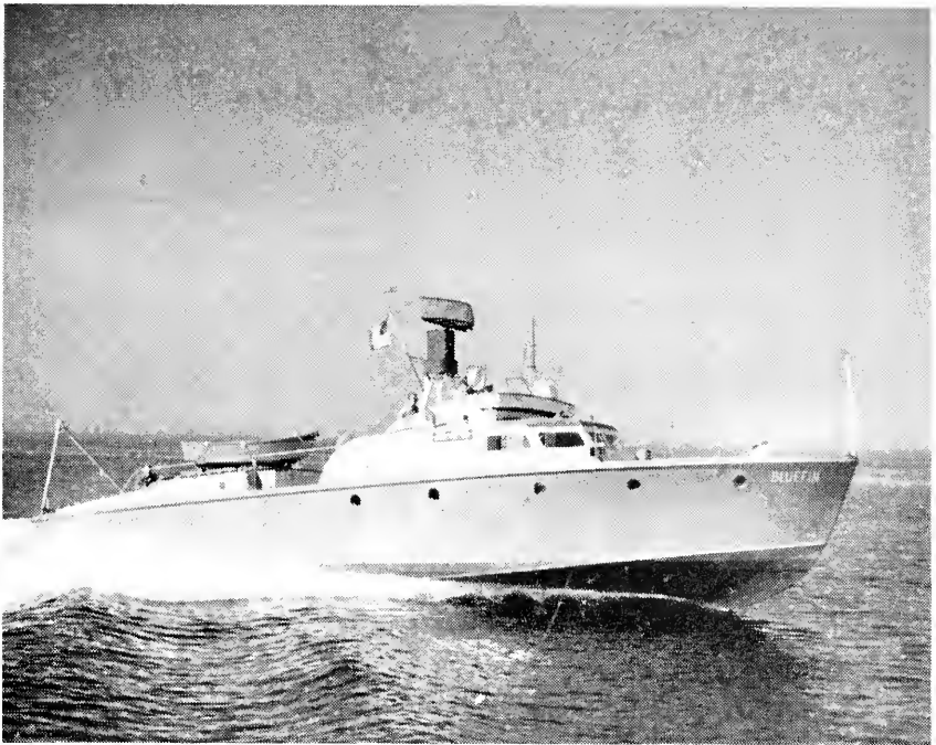
FIGURE 20. 63-foot Fish and Game patrol boat BLUEFIN. The commission operates two of these vessels in Southern California waters. Equipped with two 630-h.p. Hall Scott Defender engines, radar, radio and full marine equipment. Photograph by Vernon M. Haden, San Pedro.
