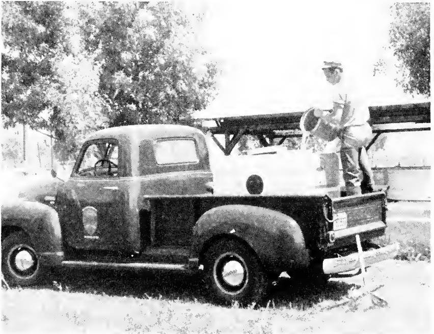
FIGURE 16. Loading trout for stocking. The pickup truck is equipped with a recently developed 150-gallon aerated planting tank. Photograph by Kramer Adams.
