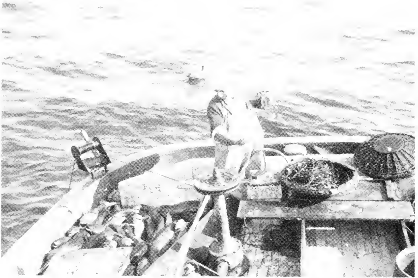
FIGURE 12. Fishing for sablefish. Hauling in a long line from a depth of 400 fathoms, with the aid of a line puller. Photograph by J. B. Phillips, Monterey, California, March 1, 1950.
