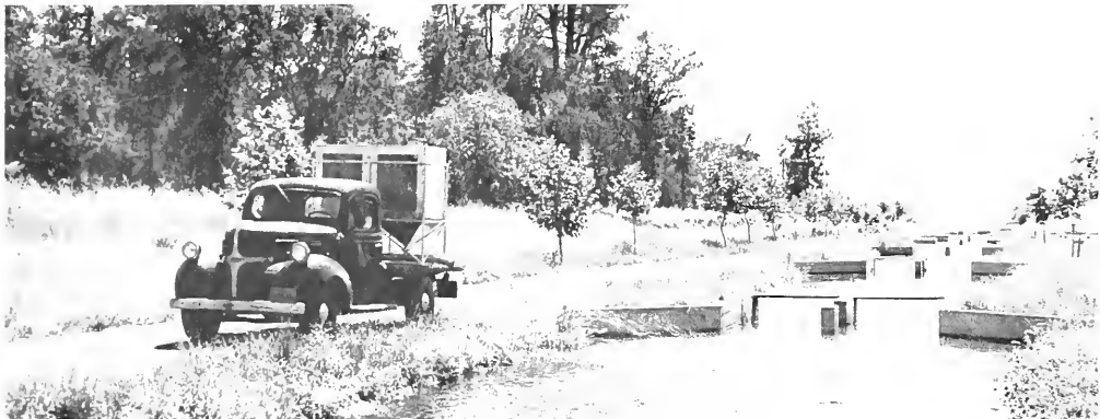
Pellet blower for blowing fish food pellets into raceway ponds provides better distribution of food and reduces time required in feeding.
