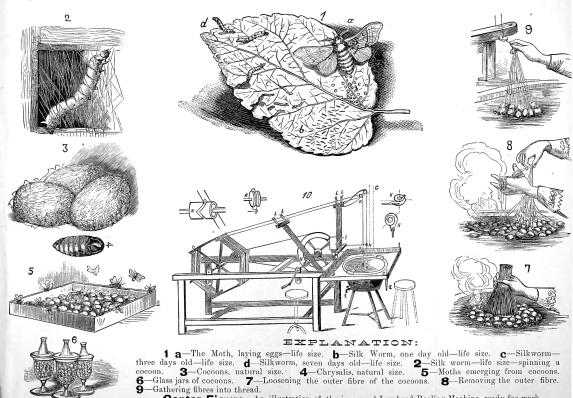
Center Figure—An illustration of the improved Lombard Reeling Machine, ready for work.
