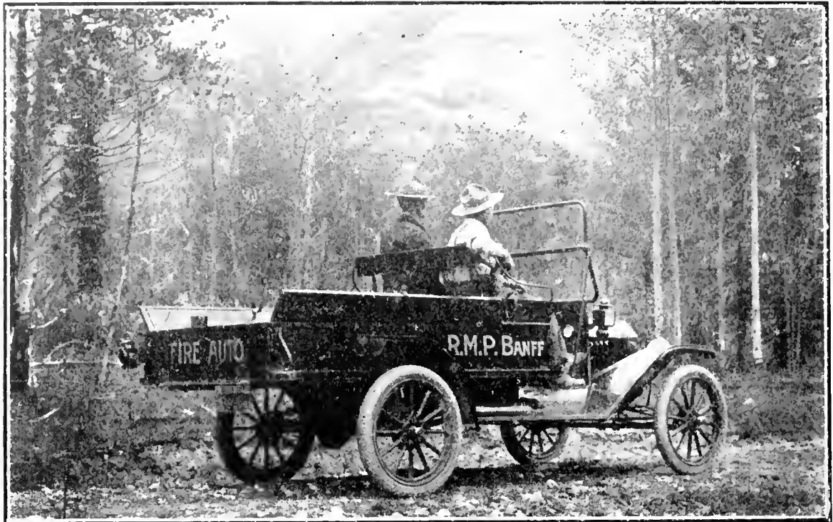
Fire Automobile in Rocky Mountains Park, Banff, for transporting portable fire pump, hose and other tools.
