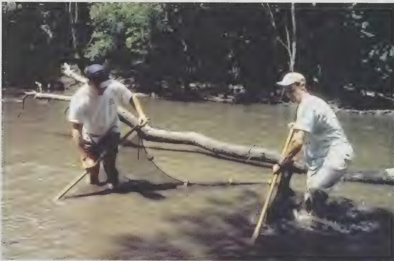
Figure 9.6. Sampling a wadable stream with a minnow seine. Minnow seines such as this one have been used to sample fishes for over 120 years and will likely continue to be used well into the future given their simple design and effectiveness. Photo by T. Rice.
