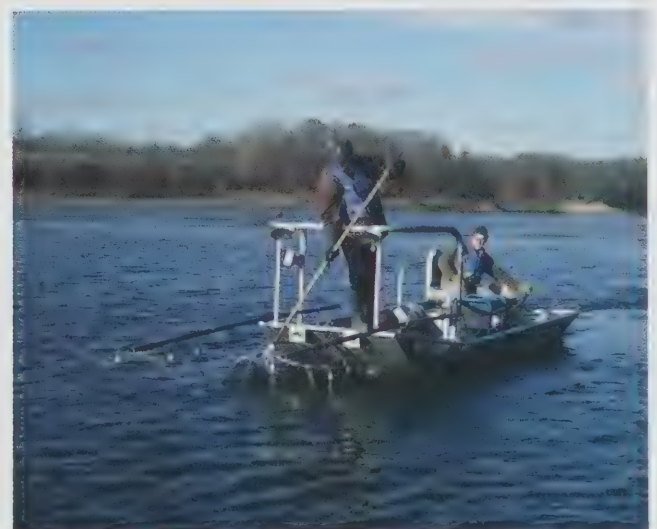
Figure 11.16. Matt Diana (front) and Dave Wahl (back) of INHS operating modern electrofishing boat on Lake Shelbyville.
