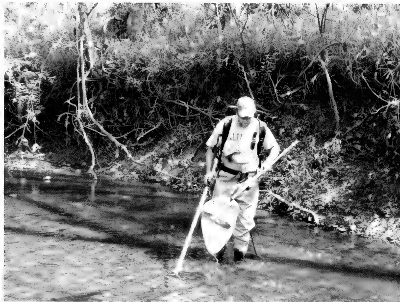
Figure 9.7. The use of back-pack electrofishers such as this one is a sampling method that has only recently become available to biologists. Photo by R. Hopkins.
