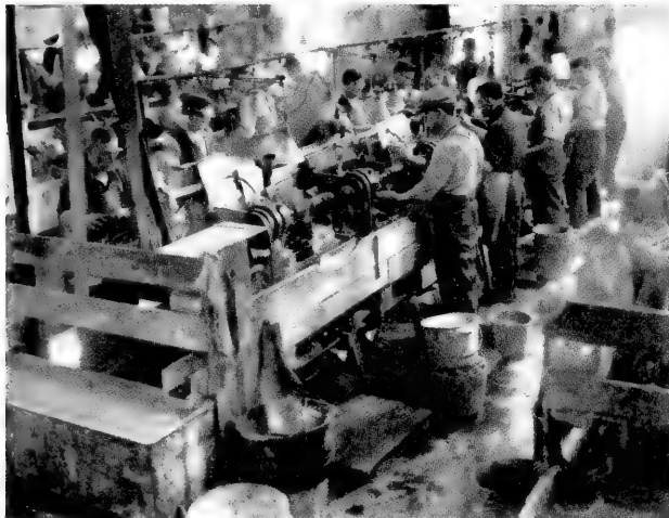
Figure 10.11. Workers use cutting machines to drill blanks for pearl buttons, circa 1910. Photo from U.S. Bureau of Fisheries.
