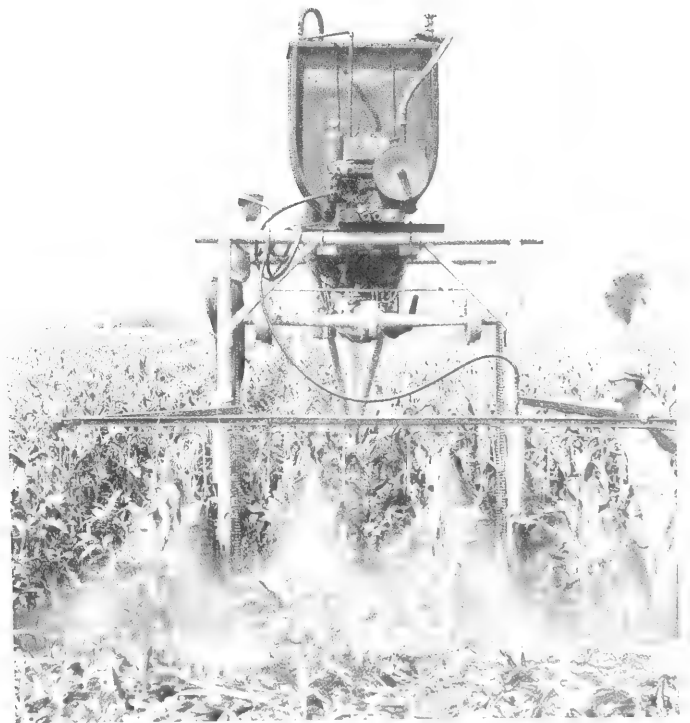
Figure 7.4. Insecticide sprayer designed by INHS entomologists and used to control European Corn Borer ( Ostrinia nubilalis ) in sweet corn, ca. 1943.
