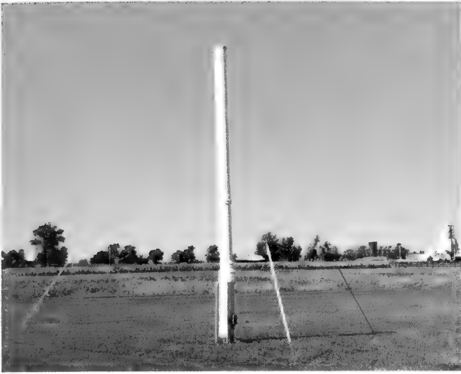
Figure 7.13. Suction trap used to monitor spread of the Soybean Aphid (photo by D. Voegtlin).
