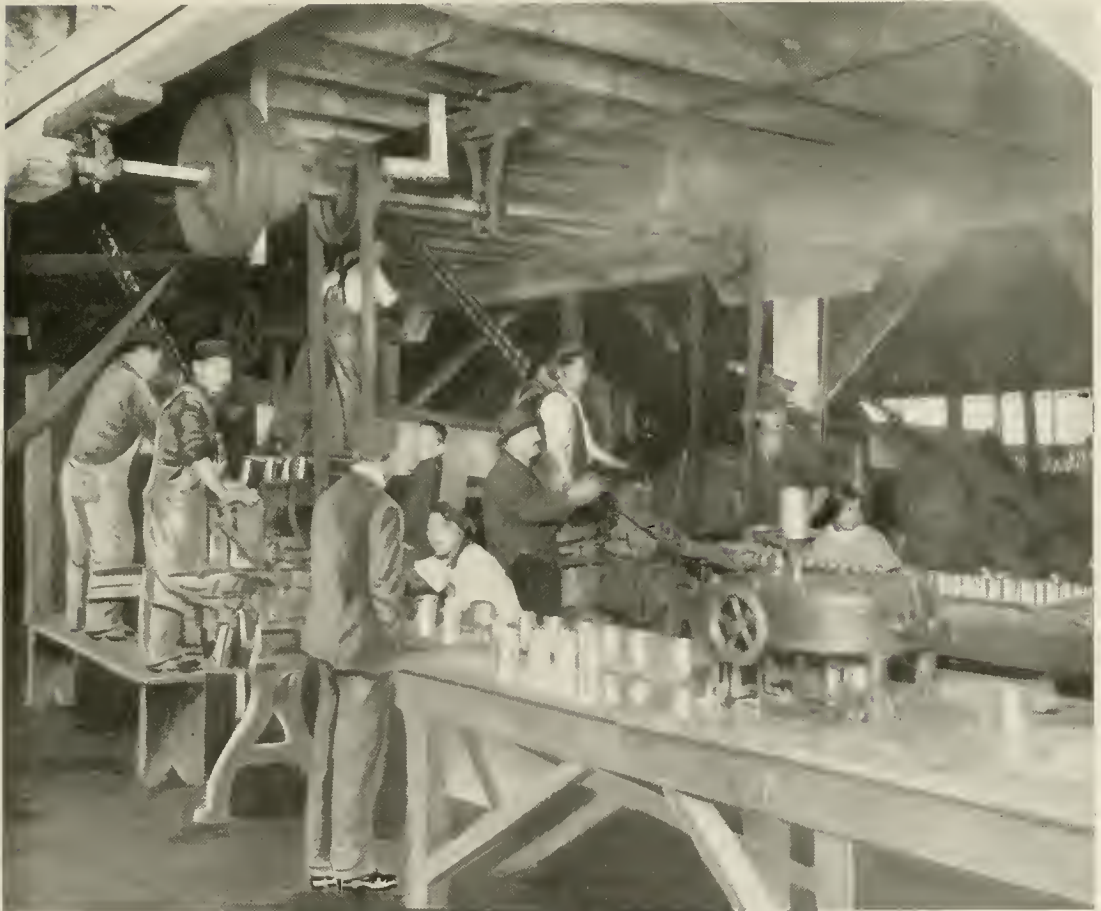
THE SALMON FILLING AND WEIGHING MACHINES.
