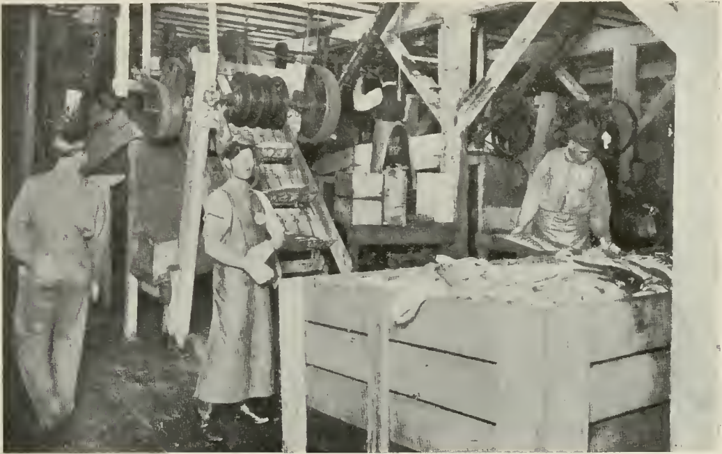
MACHINE FOR CUTTING SALMON INTO LENGTHS TO FIT THE SIZE OF CAN USED.
