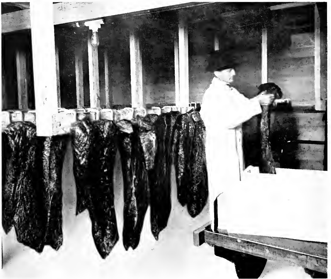
PACKING WHALE MEAT IN COOLING ROOM FOR PURPOSE OF REMOVING ANIMAL HEAT BEFORE CANNING.
