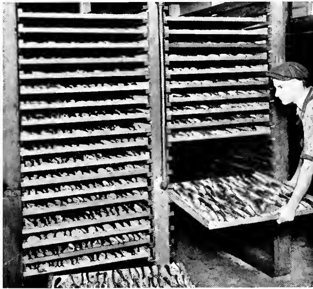
DRYING SARDINES BY ARTIFICIAL HEAT.
