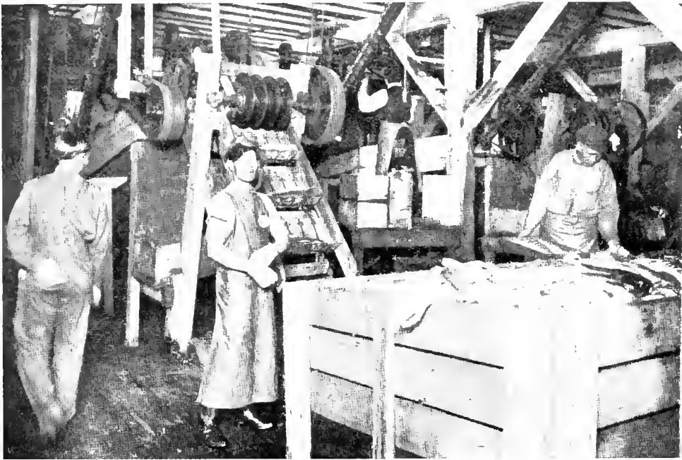
MACHINE FOR CUTTING SALMON INTO LENGTHS TO FIT THE SIZE OF CAN USED.
