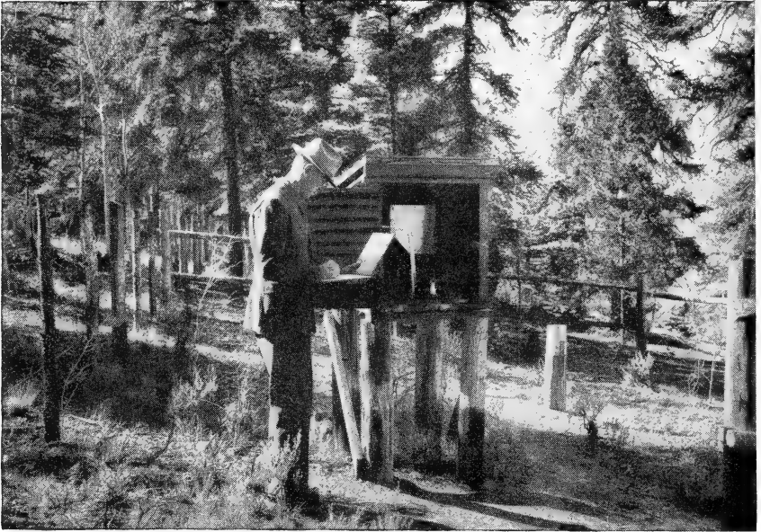
Figure 4.—Forest officer checking weather data for fire-danger. This information enables him to forecast the possibility of forest fires and to make the proper preparations. F-388144
