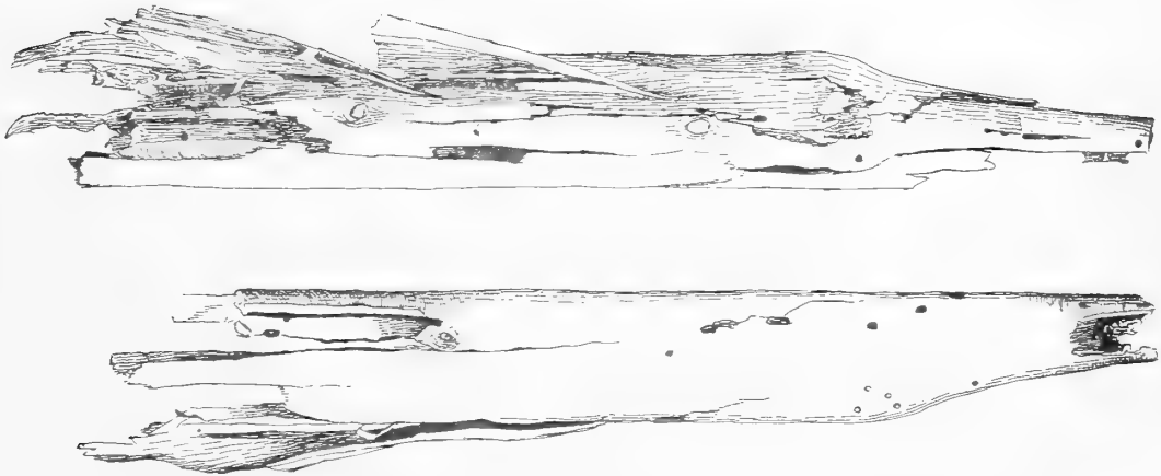
Fig. 3.—Destruction by termites of a susceptible rung, which, covered with caning, forms part of the seat of a chair whose other members are made of mahogany.
