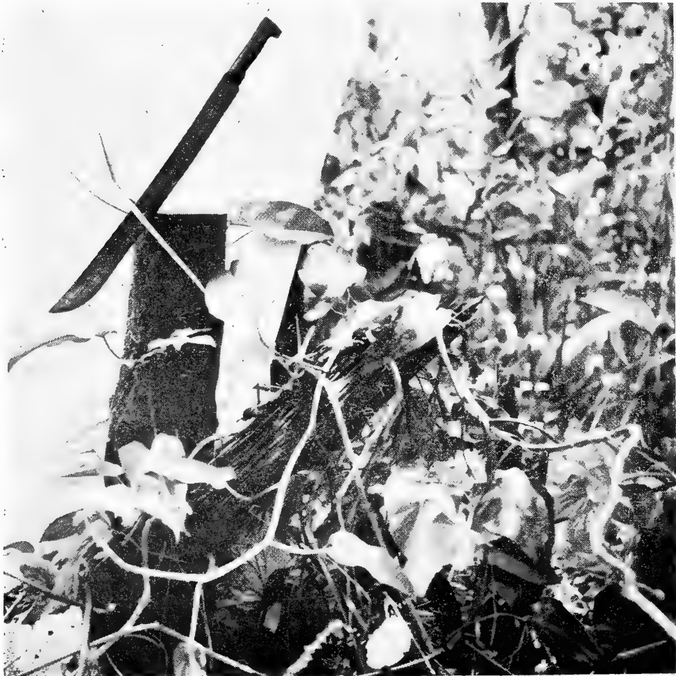
Figure 2. Post of Casuarina 18 years after treatment with Carbolineum, set in forest with high humidity and more than 100 inches annual rainfall.
