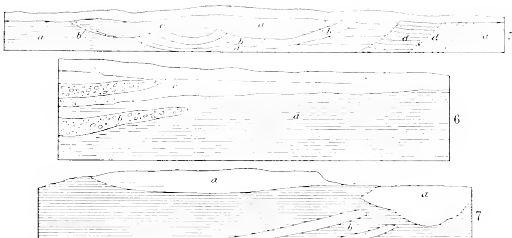
FIG. 5.—Section in cut along the Wichita Falls and Northwestern Railway, 3.5 miles south of Burkburnett, Wichita County: a , red shale; b , cross-bedded sand; c , erosional unconformity; d , alternating layers of silt and sand. (From Udden.)
