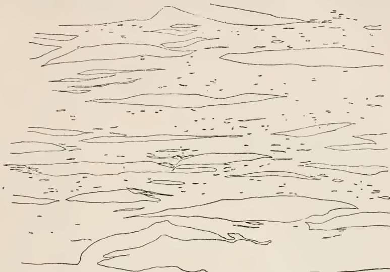
FIG. 7.—Longitudinal section of an agar plate dried at 70° C. without superficial shrinkage, with development of elongated spaces or cavities which are found when the film is hydrated. Drawn with camera lucida by Miss C. L. Carey. \times 78.5 diam.
