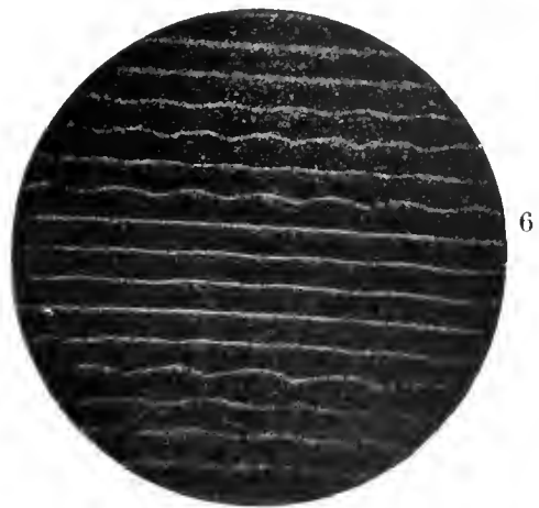
FIG. 4.—Gramophone recorder, front view. FIG. 5.—Casting from phonograph grooves. FIG. 6.—Gramophone grooves.
