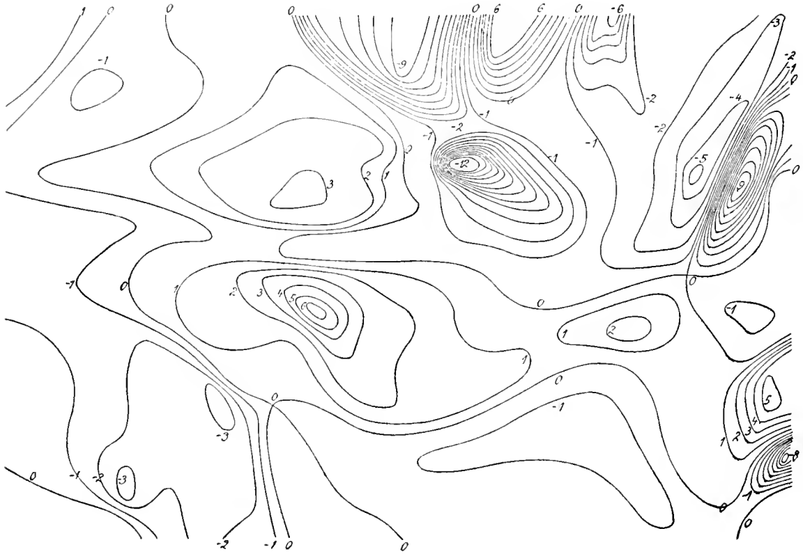
FIG. 107.—Derivative \frac{\partial v}{\partial s} of velocity with respect to the lines of flow. U. S. A., 1905, Nov. 28, 8 a. m.
