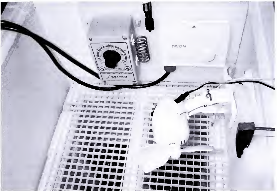
Figure 2: The control panel of the growing chamber.
