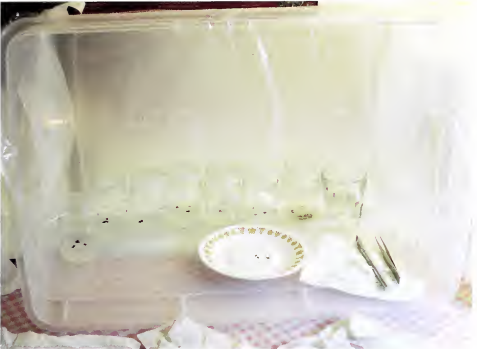
Figure 3: A simple cleanbox or transfer hood.
