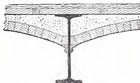
Fire-Proof Construction.—Fig. 2.—Showing Method of Using Deep Beams. The Arches may be Supported on Angle Irons Riveted to the Web of the Beams.
