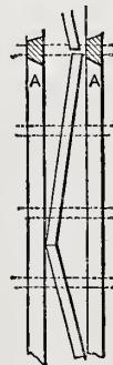
Middle-Age Roofs.—Fig. 9.—Plan of Wall Plates of Fig. 7, showing Method of Strutting.
