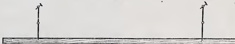
Straight Edge in Shingling, as Employed by E. S. C.
