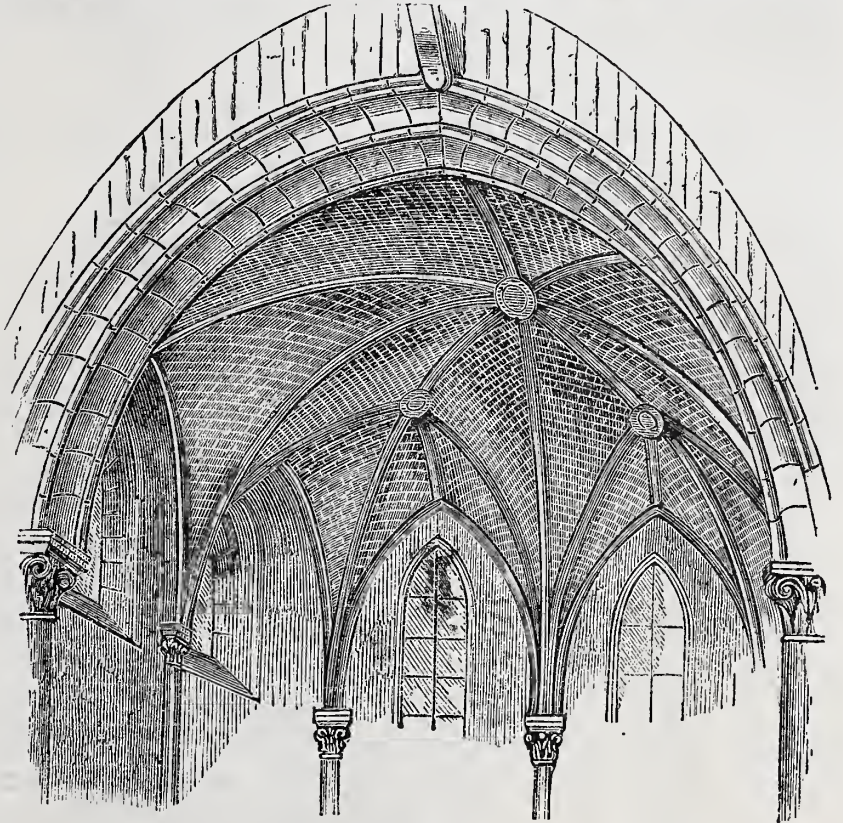
Vaults and Groins.—Fig. 10.—Vaulting of the Church of Moulherne, Saumur, France.—An Example of the Combination of Two Systems.
