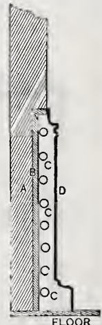
Hot Water Heating.—Fig. 3.—Base Screen, Fastened to Walls with Screws.—Pipes are Shown back of the Screen, and in End View. A, Wall. B, Paper and Iron Lining. C, Pipes. D, Face of Screen.
