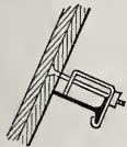
Fire-Proof Construction.—Fig. 11.—Another Method of Securing Slate. Wrought-Iron Countersunk Bolt and Hook Hanging to Purlin.
