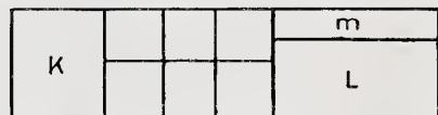
No. 4.—K, Gimlet Bits. M, Bevels. L, Hammers. Small Apartments for Screws, Brads, &c.
