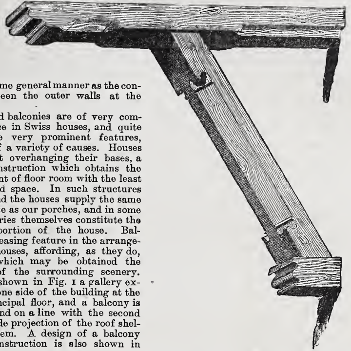
Swiss Architecture.—Fig. 8.—Example of Bracket Supporting Ends of Purlins.—From House in Canton of Berne.
