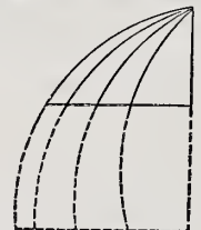
Groins, Pendentives and Niches.—Fig. 22.—Elevation of the Cradling of a Niche which is Semicircular in Plan and Segmental in Elevation.
