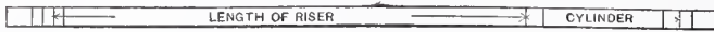
Straight Flight of Stairs with Cylinder.—Fig. 1.—Divisions of the Space Between Timbers Upon a Dimension Rod.
