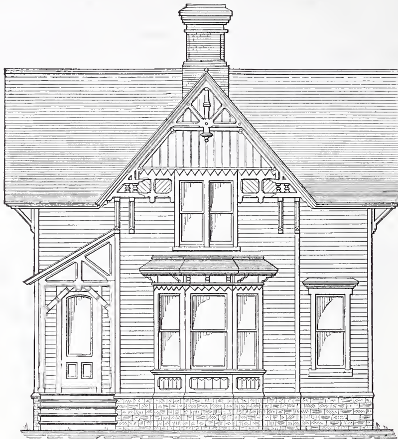
Frame Cottage.—Fig. 1.—Front Elevation.—T. I. Lacey, Architect, Binghamton, N. Y.—Scale, 1/8 Inch to the Foot.
