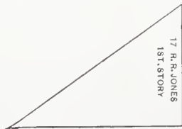
Straight Flight of Stairs with Cylinder.—Fig. 3.—Face of the Pitch Board and the Manner of Marking it.
