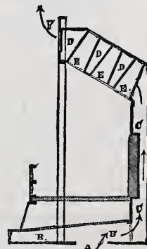
The Warming and Ventilation of Dwellings.— Fig. 2.—Vertical Section through the Jackson Ventilating Grate.
