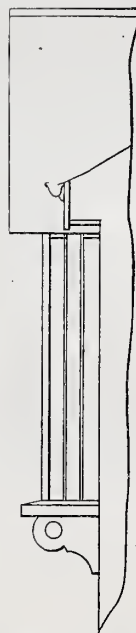
Small Frame Dwelling. —Fig. 15.— Vertical Section through Eave Cornice, and Side View of Window above Front Door. —Scale, 1/2 Inch to the Foot.
