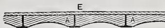
Fire-Proof Construction.—Fig. 14.—Method of Constructing Flat Roofs by Means of (A) Burnt Clay Tile Resting on T Irons. E, Layer of Cement.
