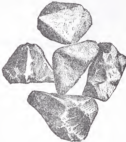
"Sharp" Sand and Quicksand.—Fig. 2.—Grains of Good Building Sand Highly Magnified.—From a Photograph.
