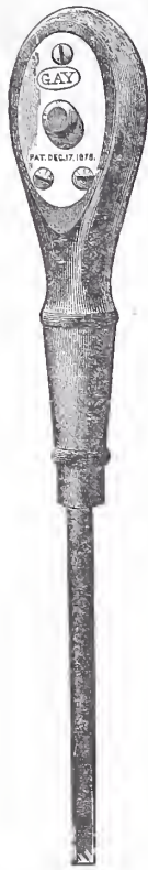
Novelties.—Fig. 1.—Gay's Ratchet Screw-Driver.
