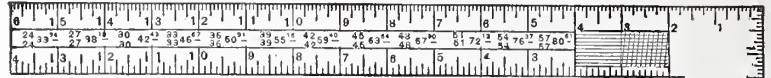
The Steel Square.—Fig. 2.—Reverse of Square known to the Trade as No. 100.
