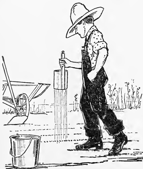
FIG. 631. — Tin Can Garden Sprinkler
