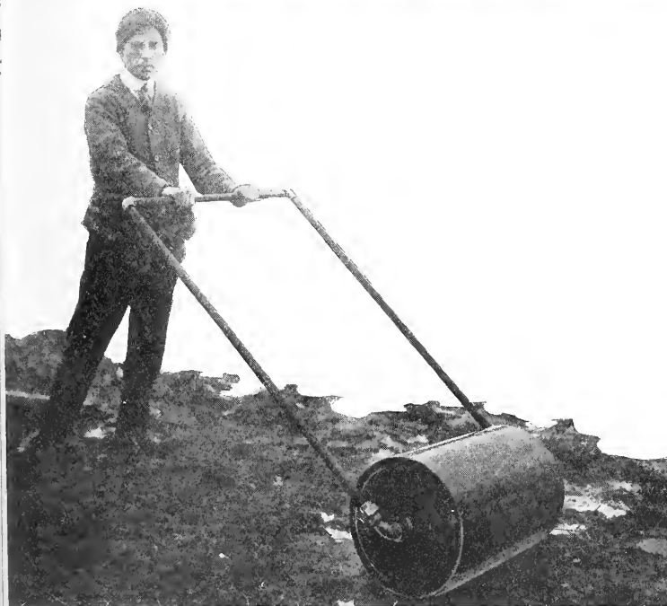
Fig. 658.—A CONCRETE LAWN-ROLLER (See Chapter 34).
