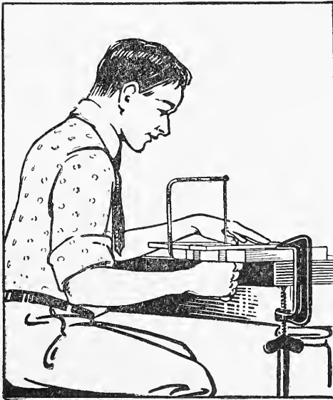
FIG. 21. — Correct Method of Using the Bracket-Saw
