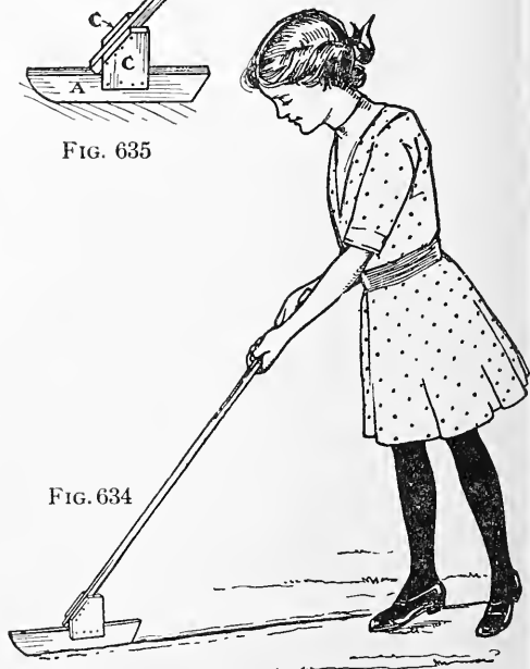
FIG. 634. — Using a Planting Trencher FIG. 635. — Detail of Trencher
