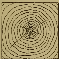
Fig. 169.—Star-shake in Balk.
