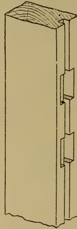
Fig. 302.—Open Mortise and Tenon Joint.
