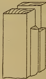
Fig. 1390.—Joint at Meeting Rail of Bottom Sash.
