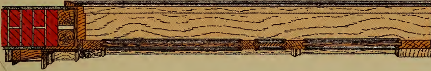
VERTICAL SECTION THROUGH DOOR
