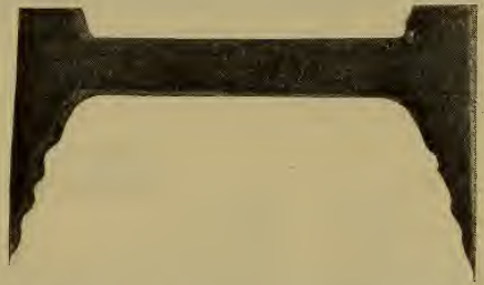
Fig. 48.—Dog made from Sheet Steel.
