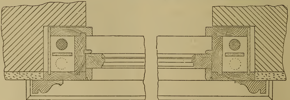
Fig. 1386.—Horizontal Section of Double-Hung Window.
