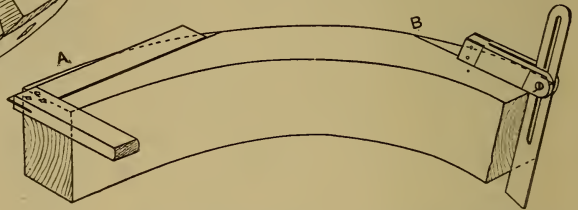
Fig. 1282.—Method of Testing Joints with Try Square and Bevel Applied to Tangent Lines.
