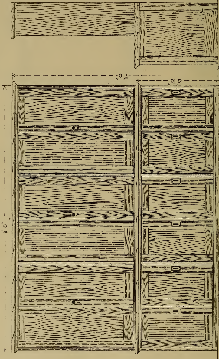
Fig. 1005.—Side Elevation of Portable Cupboard.
