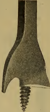
Fig. 108.—Centre Bit with Screw.
