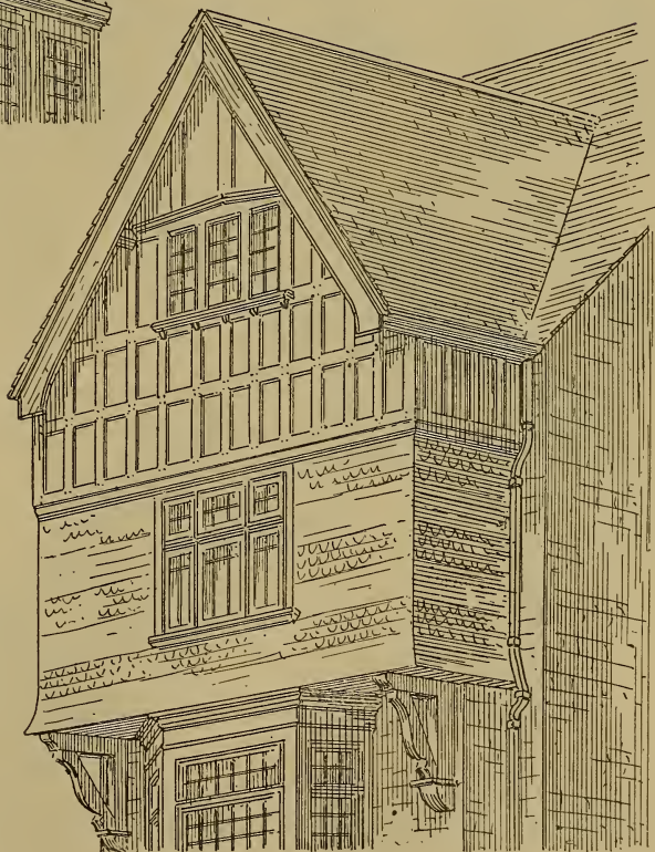
Fig. 737.—Gabled Front of House with First Floor of Timber Work Tiled, and with Upper Storey of Half-timber Work.
