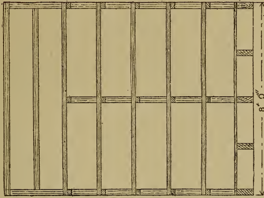
Fig. 779.—Front View of Stand for a Window.
