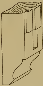
Fig. 1389.—Joint at Meeting Rail of Top Sash.
