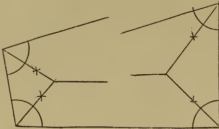
Fig. 614.—Method of Obtaining Positions of Hips.
