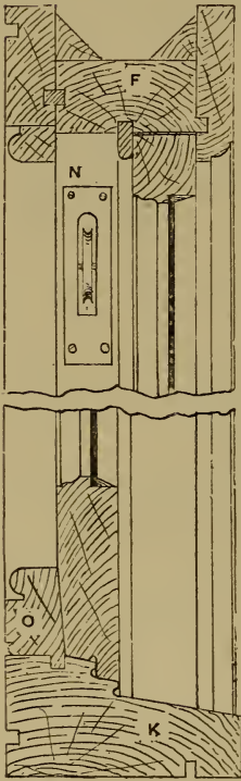
Fig. 1424.—Vertical Section through Head and Sill.
