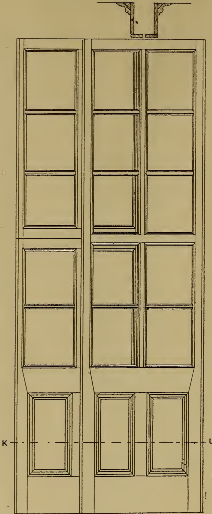
Fig. 1774.—Elevation of Door and Pieces of Framing when Folded Back to Wall.
