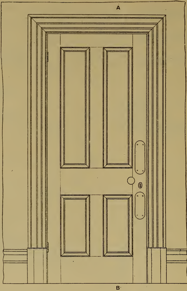
Fig. 1114.—Elevation of Four-panel Framed and Moulded Door with Linings, etc., in Partition.
