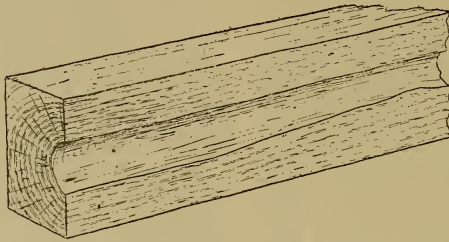
Fig. 164.—Cup-shake in Balk.
