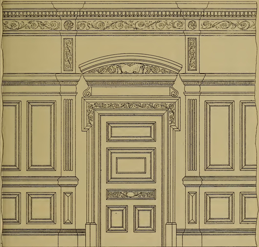
Fig. 1668.—Elevation of Door and Portion of Panelling.
