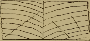
Fig. 377.— Rebated Floor Joint.
