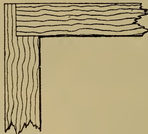
Fig. 267.—Rebated Butt Joint.
