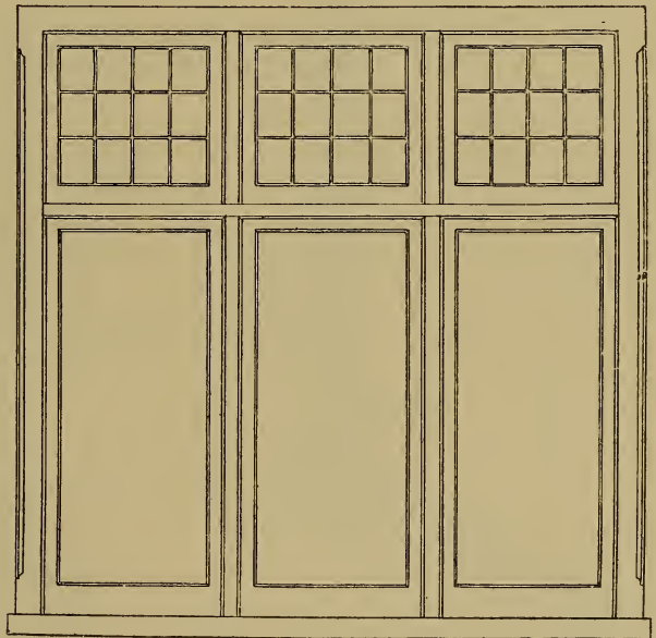
Fig. 975.—Elevation for Square Bay Window.
