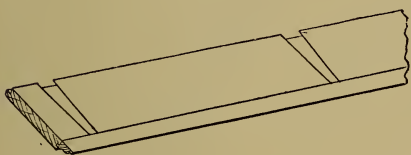
Fig. 1626.—Back of Skirting with Grooves for Fixing.
