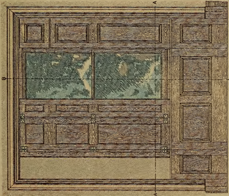
ELEVATION WITH HALF SHUTTERS CLOSED, AND HALF SHUTTER OPEN
