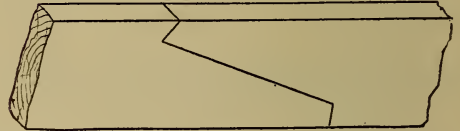
Fig. 228.—Raking Scarf used for Ridges, etc.
