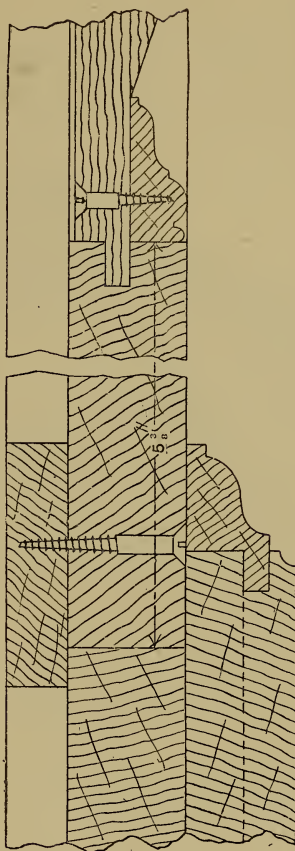
Fig. 1628.—Detail Section of Lower Part of Dado.
