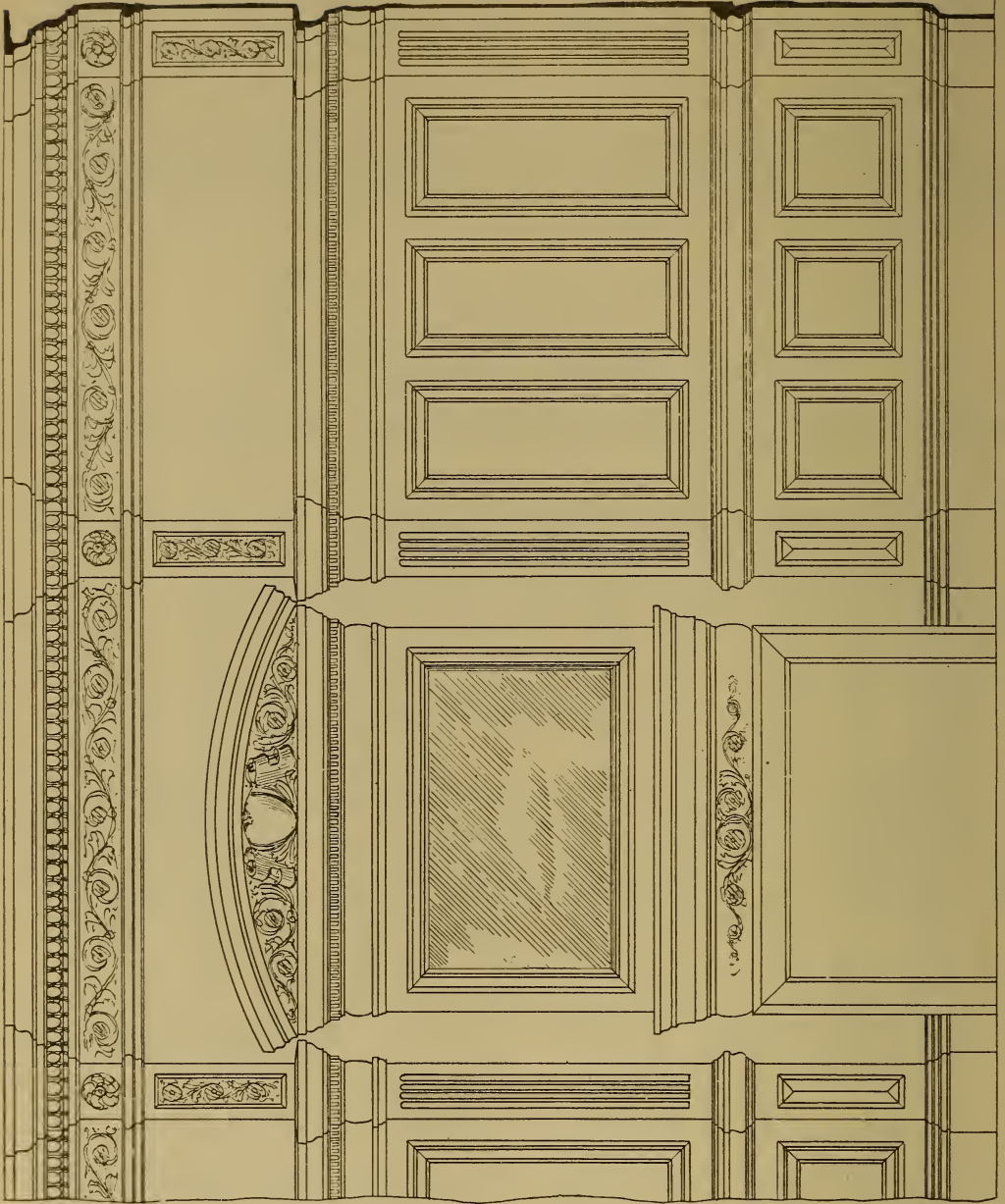
Fig. 1669.—Elevation of Mantelpiece, and Panelling Adjacent to Internal Angle of Room.
