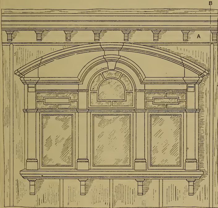
Fig. 706.—Front Elevation of completed Dormer Window and Junction of Side and Flat.
