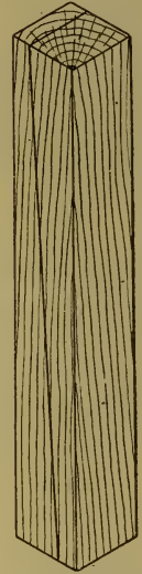
Fig. 32.—Wooden Bench Stop.
