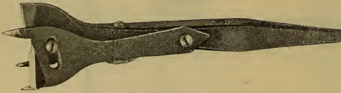
Fig. 109.—Anderson's Expanding Bit.
