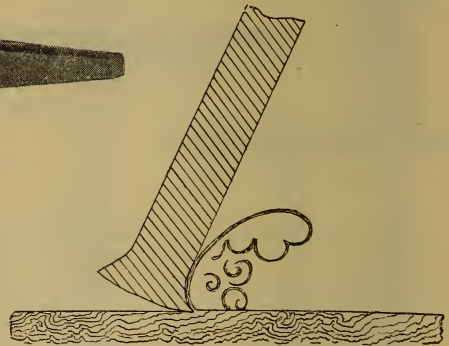
Fig. 113.—Action of Steel Scraper.
