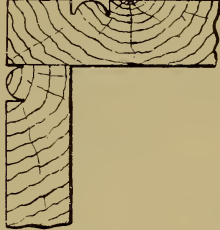
Fig. 277.— Butt Joint with Flush Beads.
