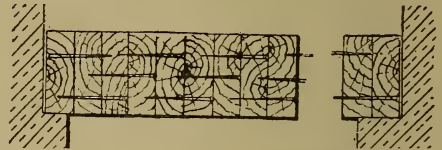
Fig. 387.—Floors of Solid Wood.
