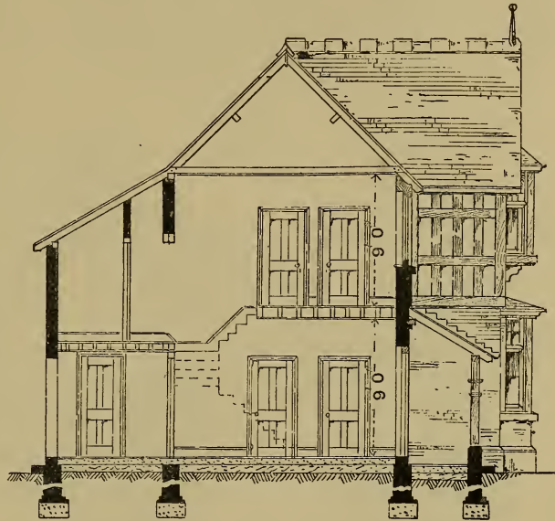
Fig. 724.— Sectional Elevation of Half-timbered House.
