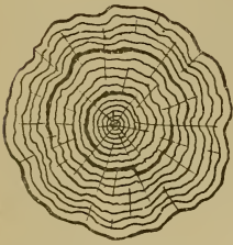
Fig. 163.—Cup-shake in Log.
