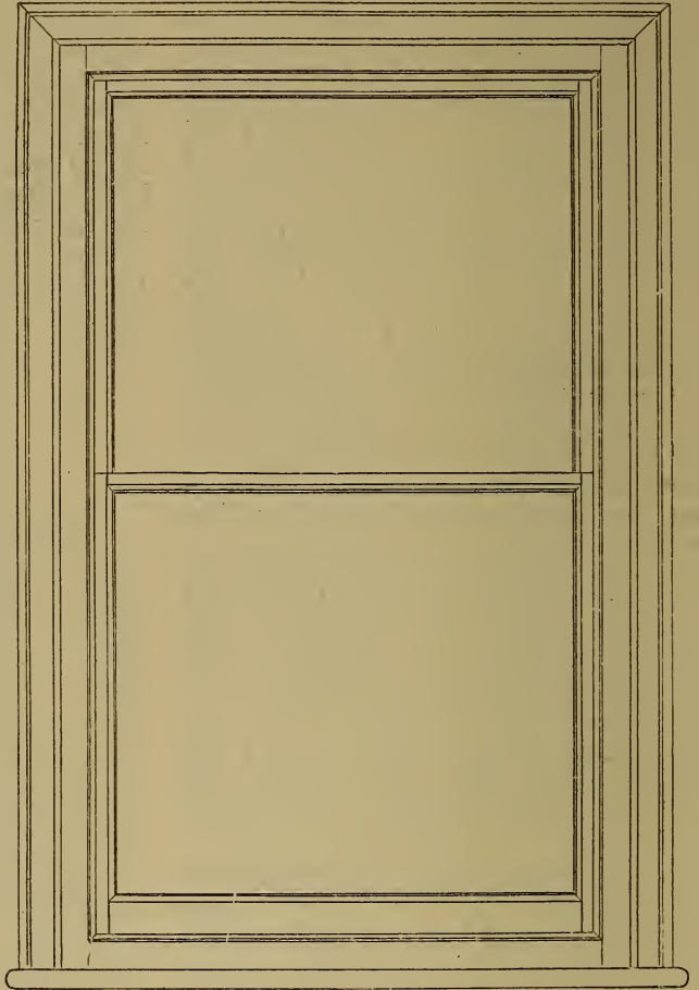
Fig. 1385.—Elevation of Double-Hung Window.
