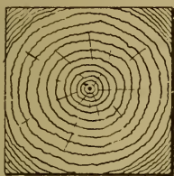
Fig. 167.—Sapwood in Balk.
