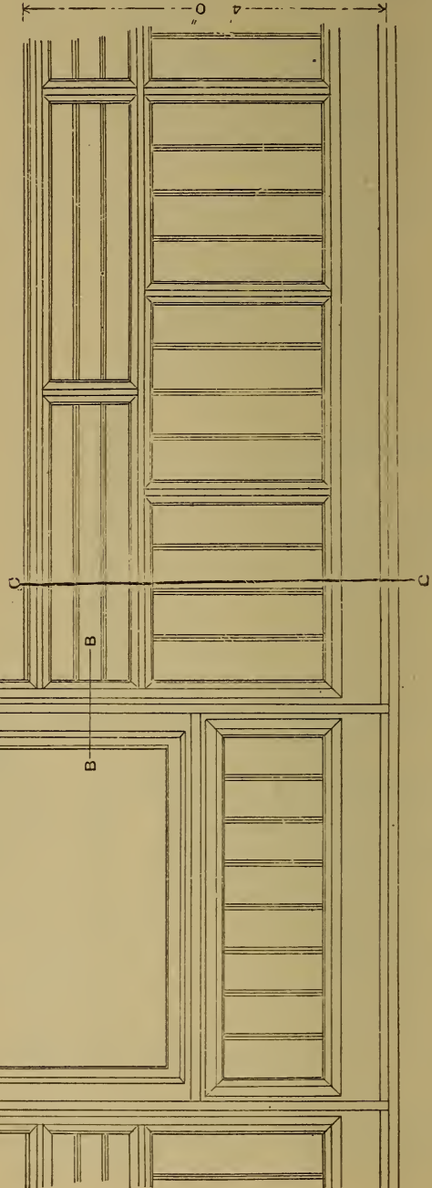
Fig. 1606.—Elevation of Sham Dado Framing with Window.
