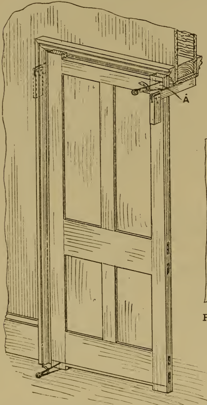
Fig. 1125.—Scribing Door for Height.
