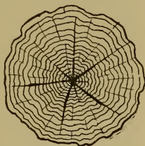
Fig. 168.—Star-shake in Log.
