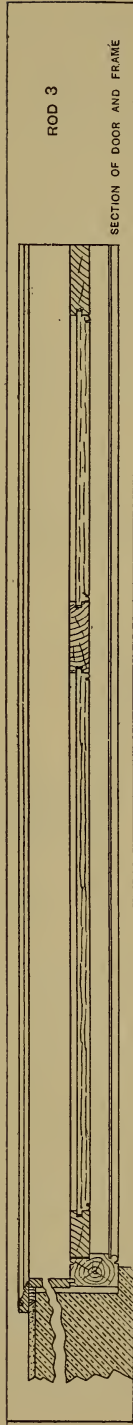
Fig. 947.—Height Rod showing Section of Four-panelled Door.
