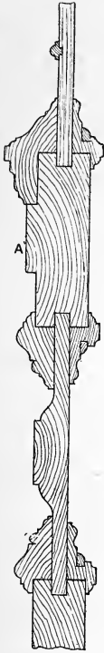
Fig. 1277.—Enlarged Vertical Section through Middle Panel and Lower Portion of Upper Panel.
