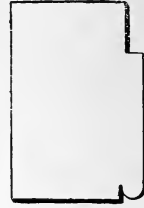
Fig. 938.—Mould of Jamb used in Fig. 936.
