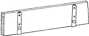
Fig. 1623.—Fixing Ground and Fillets.
