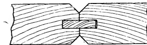
Fig. 1054.—Joints of Boarding when Ploughed and Tongued, and showing a V-joint on each side.
