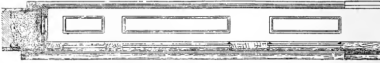
Fig. 1232.—Sectional Elevation of Door and Opening.
