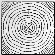
Fig. 167.—Sapwood in Balk.
