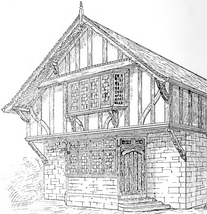
Fig. 714.—Method of fixing Door Frame in Half-timbered Work.
