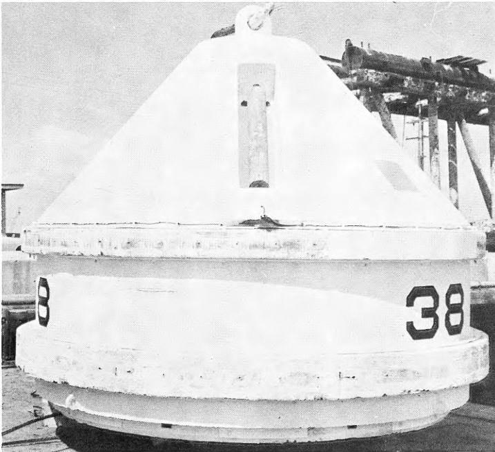
Figure 4. Inverted test buoy showing the square-foot area of bare steel on lower left of cone and location of the ground cables.
