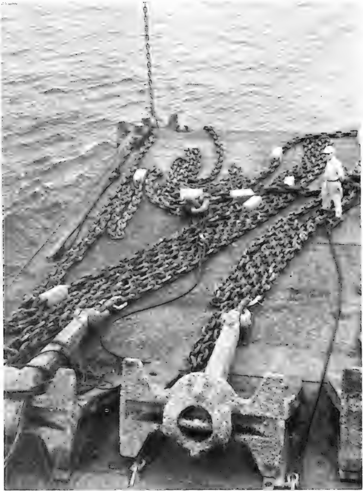
Figure 11. Ground tackle with specially cast anodes on deck of floating crane rigged for laying.
