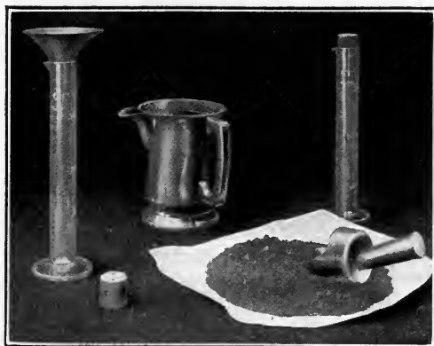
FIG. 27.—Apparatus for determining whether aggregates require washing before use.
