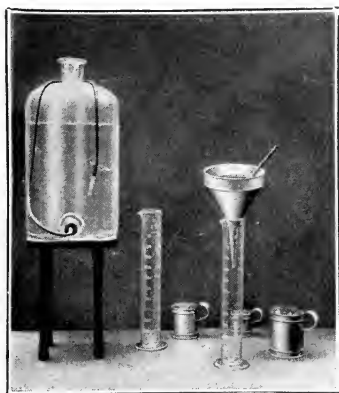
FIG. 31. — Apparatus for checking the composition of Concrete Mixtures.
