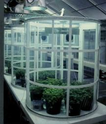
Computer controls for the CSTRs keep actual concentrations of ozone ( —) close to target concentrations ( ) and allow independent funnigations in separate chambers.
