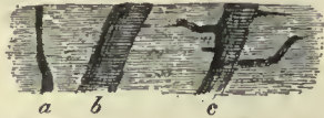
Section showing dikes traversing stratified rocks. a, b, simple dikes; c, branching dike.
