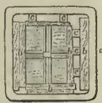
Printers' Chase. a, frame; b, d, e, furniture of wood or metal; c, a, c, quoins.
