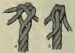
A Three-stranded Rope Crowned. a shows the arrangement of the strands before, and b after hauling taut.
