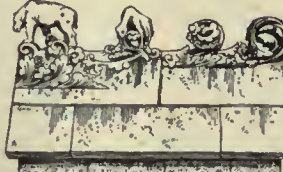
Cresting.—Butress of Notre Dame, Dijon, 13th century. (From Viollet-le-Duc's 'Dict. de l'Architecture.')
