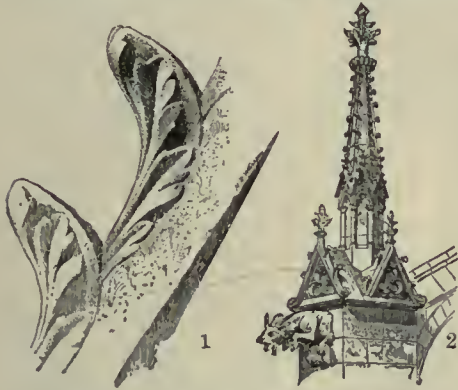
1. Crockets in detail, from Porte Rouge, Notre Dame, Paris. 2. Crockets applied on a pinnacle. (From Viollet-le-Duc's "Dict. de l'Architecture.") Both examples, 13th century.
