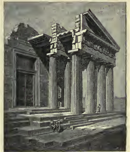
Doric Architecture.—Diagram of northeast angle of the Parthenon, illustrating method of construction.
