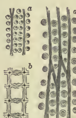
Disk-bearing Wood-cells of the Pine, magnified. a, a, longitudinal section of cells; b, cross-section of cells.
