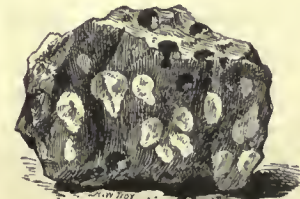
An Amygdaloid (Diabase) with calcite nodules or amygdules.
