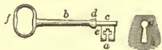
Ward-lock Key and its Keyhole. a, Main ward, or bridge; b, stem or body; c, pin; d, collar; e, bit or web; f, bow; g, eye; h, slot.
