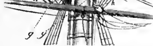
Rigging of Ship's Top. ff, top; gg, lubber's holes; A B, futtock-shrouds.
