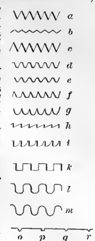
Screw-threads. a, c, V-threads; b, shallow thread; d, truncated thread; e, angular thread, rounded top and bottom; f, thread with bottom angles truncated (wood screws); g, rounded thread, sometimes used in joinery; h, thread beveled more on the inner side than the outer, by which a firmer hold against withdrawal is secured; i, German wood-screw thread; j, rectangular thread, much used in large screws; k, same as j , with truncated angles; l, rounded thread; m, special types of thread.
