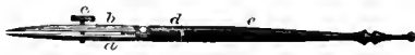
a , fixed blade; b , adjustable blade; c , adjusting-screw; d , handle, which screws into a socket at d .
