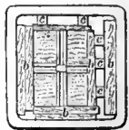
Printers' Chase. a, frame; b, d, e, f, g, h, i, j, k, l, m, n, o, p, q, r, s, t, u, v, w, x, y, z, furniture of wood or metal; c, c, c, c, quoins.
