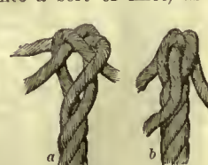
A Three-stranded Rope Crowned. a shows the arrangement of the strands before, and b after hauling taut.
