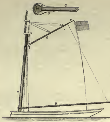
Gaff. B, boom; CC, cheeks; G, gaff; M, mast; P, peak; T, throat or jaw.
