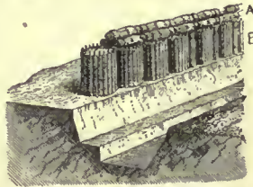
Part of Trench, with A, Fascines, and B, Gabions.
