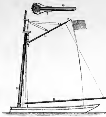
Gaff. B, boom; CC, checks; G, gaff; M, mast; P, peak; T, throat or jaw.
