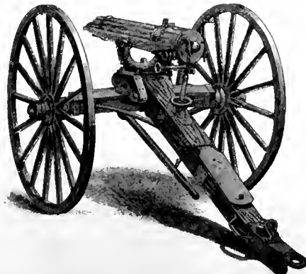
Musket-caliber ten-barrel Gatling Gun.
