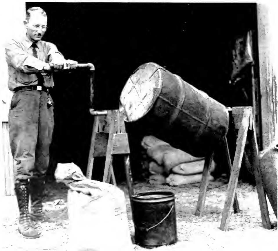
Homemade mixer used about 25 years ago by plant pathologists of the Illinois Natural History Survey to demonstrate effectiveness of chemical treatments in control of seed-borne diseases of small grains.
