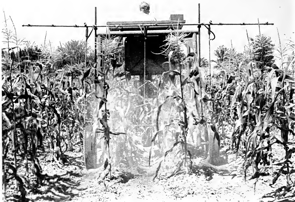
Spraying equipment developed in recent years by entomologists of the Illinois Natural History Survey for the control of the corn earworm and the European corn borer on sweet corn and field corn.
