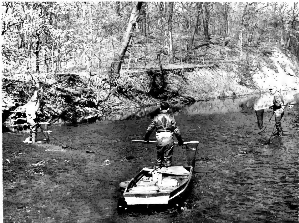
Fisheries technicians of the Illinois Natural History Survey using fish shocker for sampling the population of a stream. The shocker is a recent development that has been used successfully in both streams and lakes.
