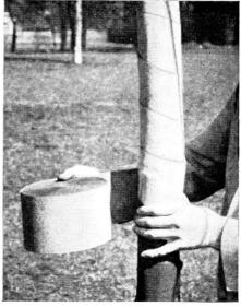
base and spiraling in opposite direction to paper. Four inches wide, in 8-inch diameter rolls containing about 155 lineal feet.
