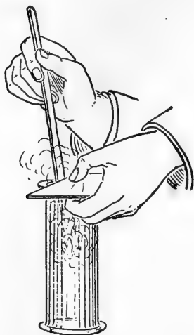
FIG. 15. — Testing oxygen with burning splinter.
