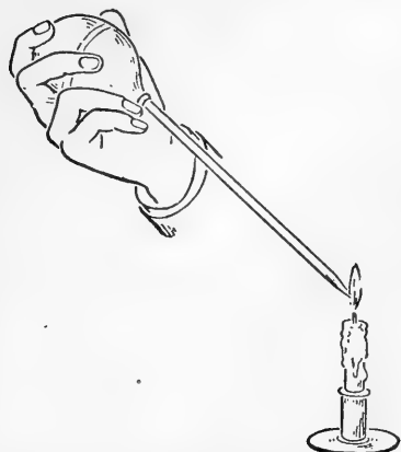
FIG. 26. — Obtaining unburned gas from candle.
