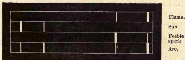
FIG 77.—Showing the various intensities of the lines of Lithium under different conditions.
