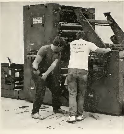
One of the printing units for the web offset is pushed into position.
