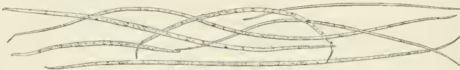
FIG. 2.—Rice-straw fibers. Though comparatively short, these are strong and felt well. (Enlarged 71 diameters.)
