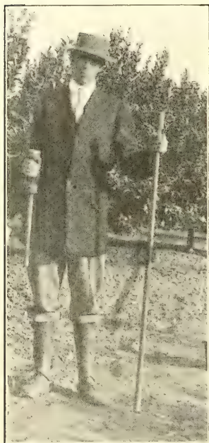
FIG. 60.—The King soil sampler is very useful for determining the downward progress of irrigation water.
