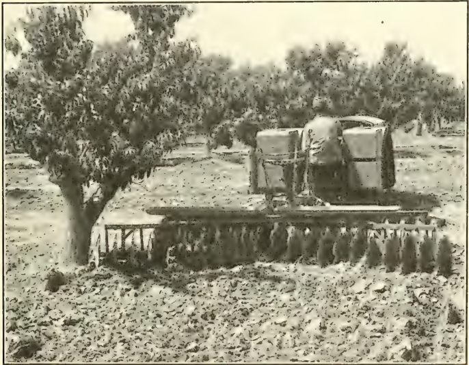
FIG. 50.—Ground under trees may be worked with ease by means of an orchard tractor.
