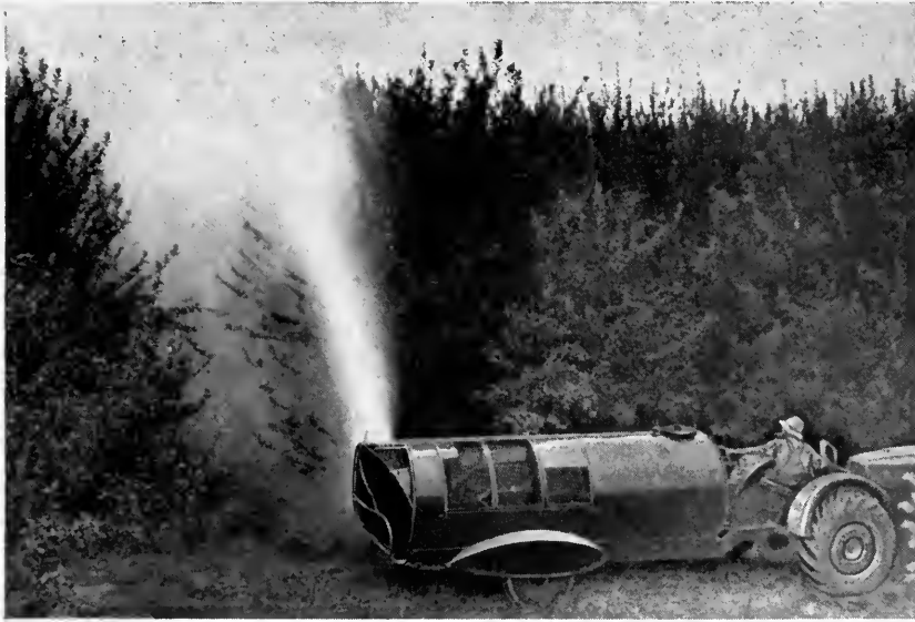
This new type of sprayer, called a speed sprayer, is especially adapted to large acreages. It saves more time and labor than the commonly used sprayers and sprays all trees alike. Fig. 7
