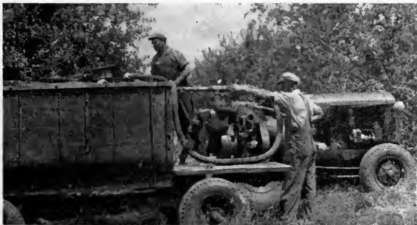
In Orchard 9 a conveyor was used to fill the spray machine. With it, more spray was laid on per day with less labor.
