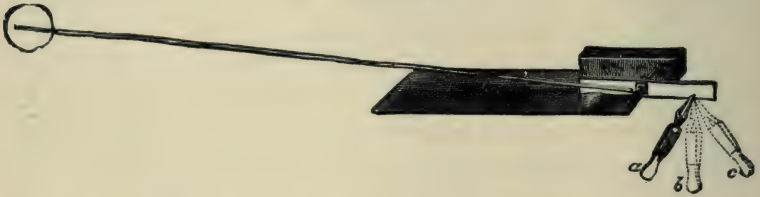
FIG. 158.—Instrument for showing the Action of Heat and Cold and of Poisons on the Frog's Heart.
